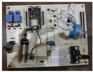
Gambar 2. Trainer sistem mikrokontroler NodeMCU ESP8266 V5 berbasis Internet of Things (IoT)
