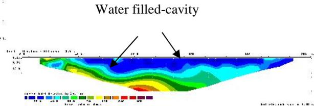
Figure 11. Resistivity section of Line 6
