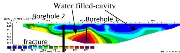
Figure 9. Resistivity section of Line 4
