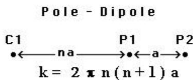
**Figure 3.** Pole Dipole array (Loke,M.H., 1999)
