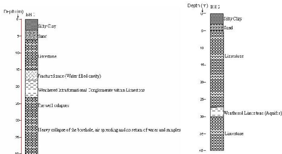
Figure 12 The lithological log of Borehole 1 and Borehole 2
