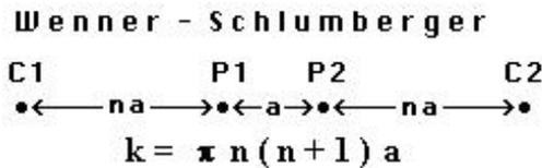
**Figure 2.** Wenner Schlumberger array (Loke,M.H., 1999)
