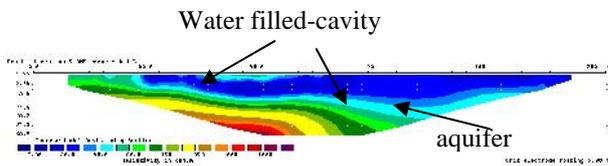
Figure 7. Resistivity section of Line 2
