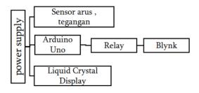
Gambar 1. Blok diagram
